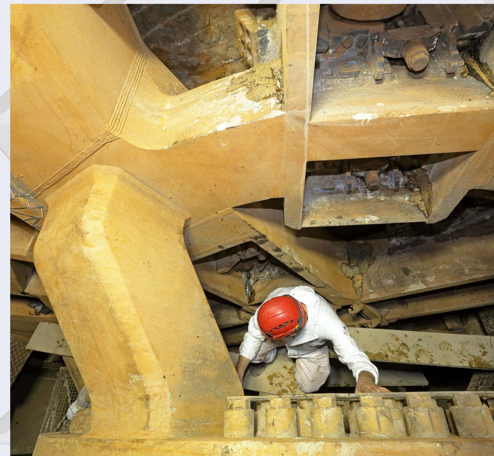
Maintenance works inside TBM "ATHENA" excavation chamber.
