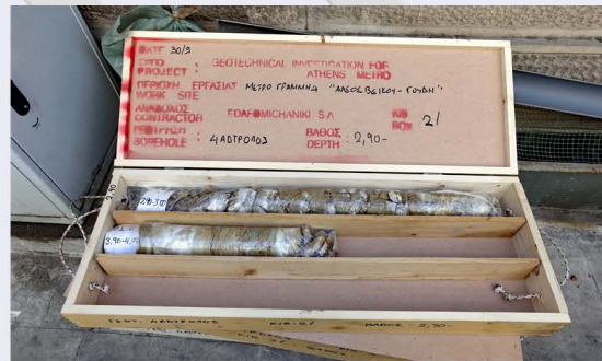
Borehole samples from Kypseli Station.
