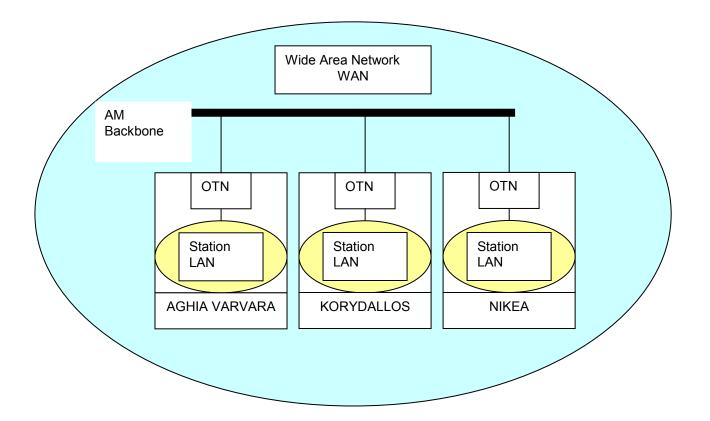
The LAN local networks of the stations communicate via the Metro's WAN. The coupling between the LAN and the WAN is ensured through OTN.
