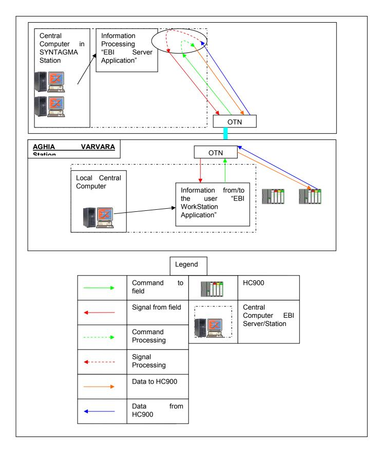
For example, if the user activates a fan from the graphics mask, the command will be transferred through to the EBI Server in SYNTAGMA Station, where all necessary actions are performed, before it is transferred to the HC900 controllers of the station. The data to update the graphics and to notify the user on the result of his action shall equally derive from the EBI Server of SYNTAGMA Station.
