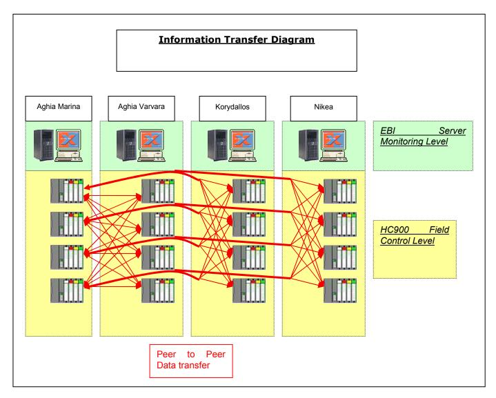
Communication between HC900 controllers is ensured via Modbus Peer to Peer communication.
