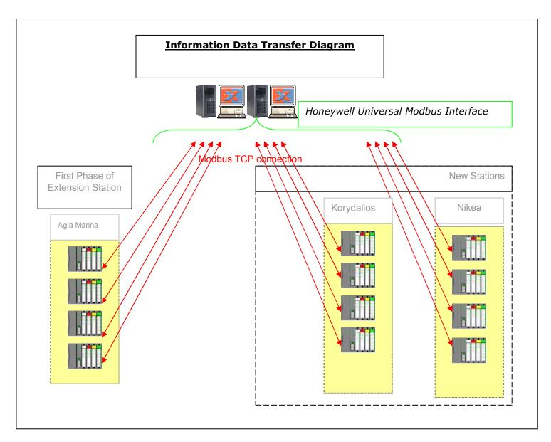
We should stress that the EBI Server at Syntagma operates the same way as the EBI Server local systems; the only difference is that data are transferred through the WAN network (a fact that does not affect the exchange of information). The EBI Server at Syntagma operates in parallel with the local EBI Server of each station, while these systems are equivalent and fully autonomous and independent.
