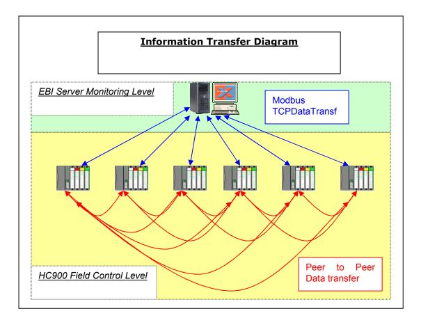
The above diagram depicts how information is transferred to the system. HC900 controllers communicate via peer-to-peer communication irrespective of their location in the physical network (as shown on the aforementioned diagram for the first HC900 controller). They all carry information directly, also irrespective of where they are located in the physical network, to the EBI Server of the station via Modbus TCP protocol.
