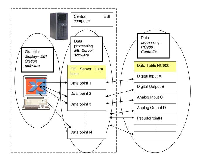
The workstation can communicate with both EBI Servers (SYNTAGMA Servers and local station Servers) of the Metro network which collect information and control the equipment of the local station. More precisely:
