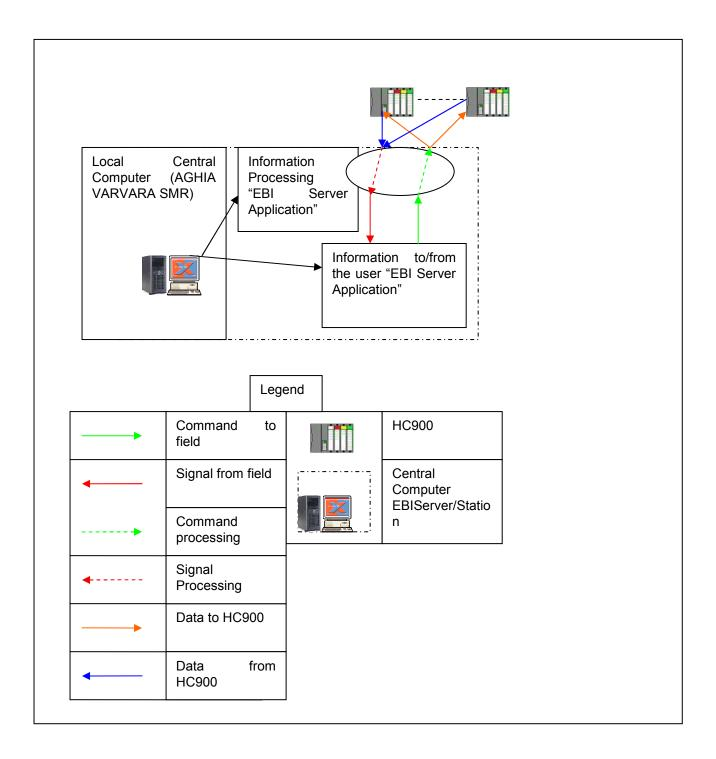
• the workstation operates as a workstation of the Redundant EBI Server of SYNTAGMA Station and information flow is ensured through the WAN.
