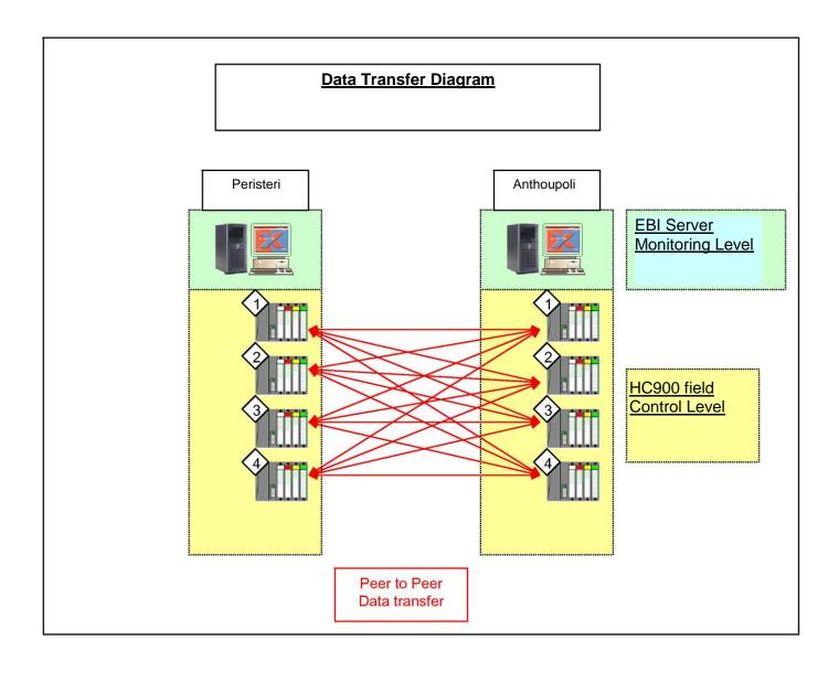
It is worth observing on this diagram that it depicts a network where the phase of the extension to which a station belongs does not play a role, which provides the option for data exchange between Peristeri to Acropoli Station and vise-versa. This is in essence a communication among the HC900 controllers of different stations, as analyzed in paragraph 3.3.2 (precisely the same operation with two adjacent stations belonging to phase A extensions, e.g. Sepolia – Agios Antonios).
