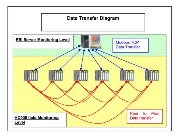
The above diagram presents the data transfer method in the system. The HC900 controllers communicate with each other via PEER-to-PEER communication, irrespective of their physical location on the network (as shown in the above diagram for the first HC900 controller). All controller directly transmit data, irrespective of their physical location in the network, to the EBI Server of the Station via the Modbus TCP protocol.
