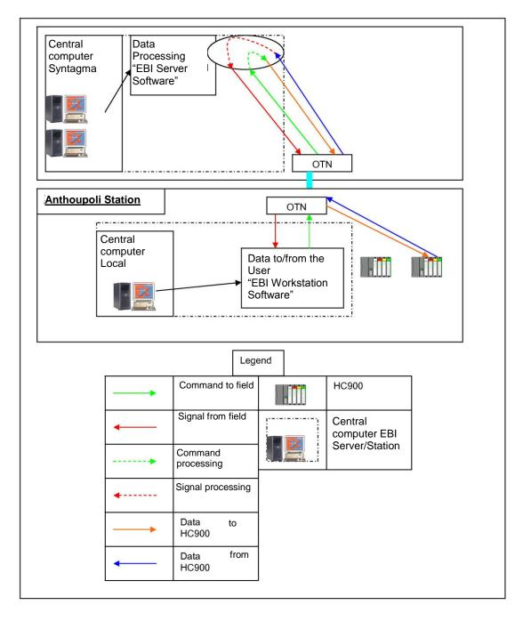
For example, when the user activates a fan from the graphic screen, the relevant command shall be transmitted via WAN to the Syntagma EBI Server, wherefrom the appropriate actions shall be implemented to transmit the command to the HC 900 controllers of the station. Similarly, the Syntagma EBI Server shall be the source of the data for graphic screen update and user warning about the effect of his action.
