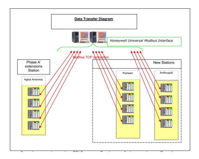
It must be stressed that the Syntagma EBI Server shall operate in the same fashion as the local EBI Servers, the only difference being that all data shall be transmitted via the WAN network (which does not affect data exchange). The Syntagma EBI Server shall operate in parallel to the local EBI Server at Peristeri as two peer systems, while the two systems shall be fully autonomous and independent.
