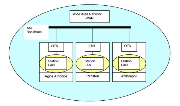
The local LAN networks of the stations communicate with each other via the Metro WAN network. The link between LAN and WAN is implemented via the OTN.
