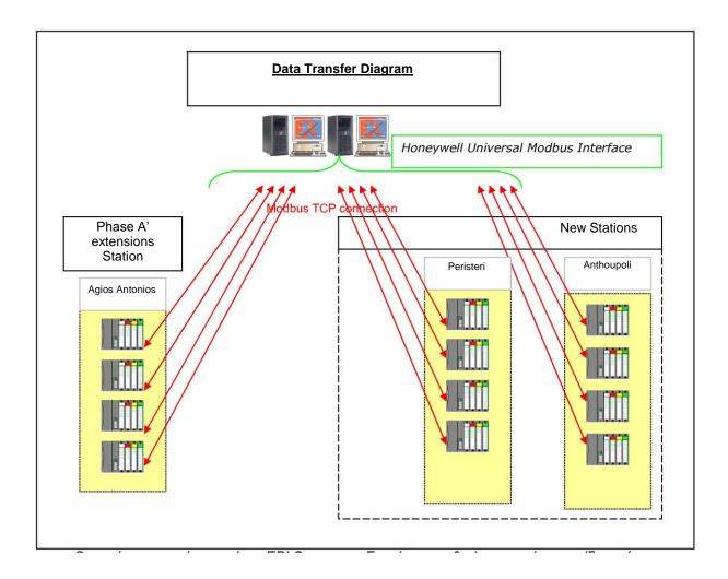
the two-way transmission of all data related to communication problems. The HC900 controllers of the new stations shall be essentially incorporated into the already operating monitoring system (EBI) as an expansion and not as a new addition, and thus nothing shall change for the OCC users as regards the monitoring and control activities for the phase A Metro extensions.
